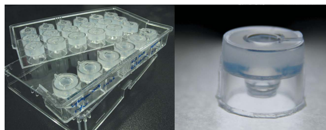
Figure 1 Inverted Cryschem plate with solidified mother liquor (left) and the outer shape of an individual well (right).
