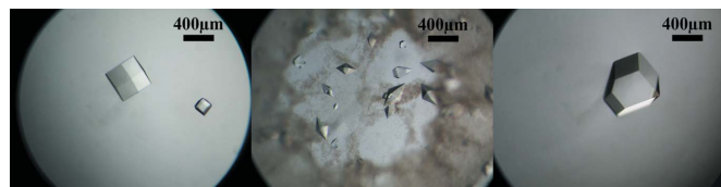
Figure 2 Crystals of hen egg white lysozyme (left), thaumatin (middle) and glucose isomerase (right) grown using the 'upside-down sitting-drop' vapor diffusion method.
