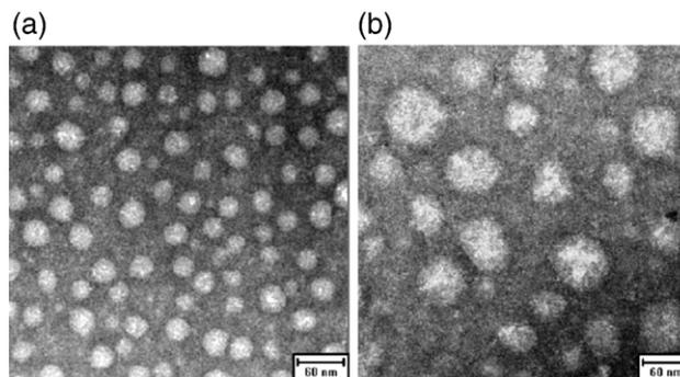
Fig. 3. Transmission electron microscopy images of (a) MPEG-HPAE and (b) DOX-MPEG-HPAE micelles.
